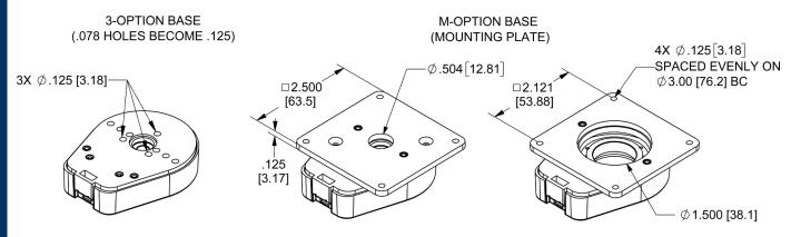
FOR SHAFTS ≤ Ø .394 [10] REQUIRES AN ADDITIONAL .125 [3.18] SHAFT LENGTH
